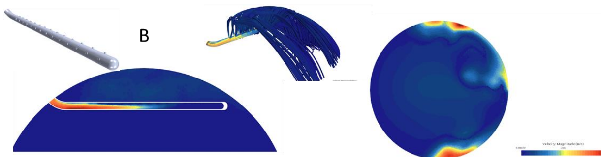
Figure 28. STARCCM+ study of configuration B steam injection
